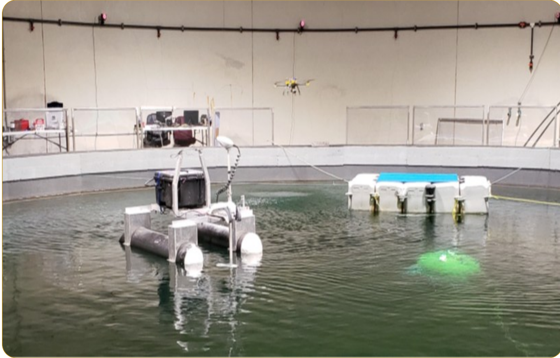
Figure 33: All 3 marine robots in the experimental validation. The USV is left in the foreground. The surfaced UUV is right in the foreground. The barge is behind both. The UAV is left of the barge. On the wall, the red LED rings are 3 of the 8 motion capture cameras installed in the Aquatron Pool tank. [6]
