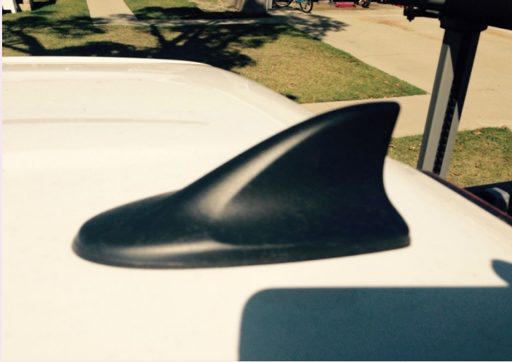
figure 2 Low Profile Shark fin antenna mounted on car*
